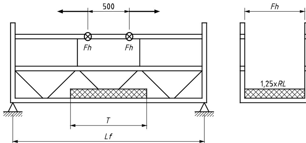
**Figure A.4 — Horizontal loads on guard rail**
