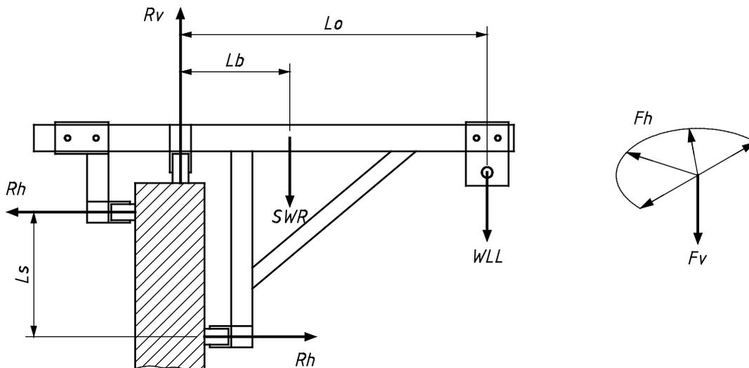
Figure 13 — Parapet clamp
