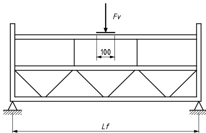
**Figure A.5 — Vertical loads on guard rail**
