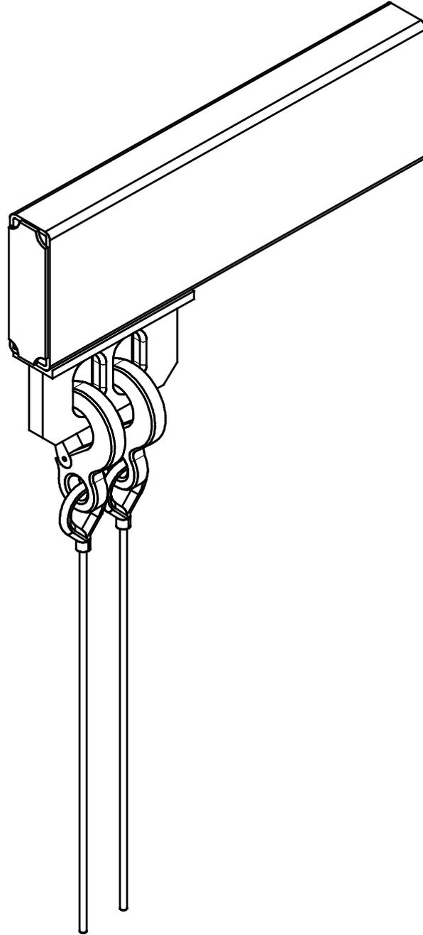
Figure 20 — Example of typical suspension points
