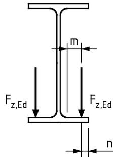
Figure G.7 — Wheel loads on bottom flange
